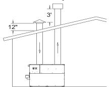
FIG. 20 Vertical DirectAire Installation with Roof Top Combustion Air Inlet
